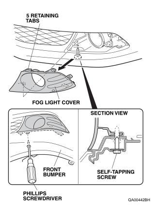
2. Remove the fog light from the front bumper (two self-tapping screws and unplug the connector).
