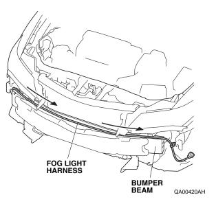
32. Secure the clip on the fog light harness to the vehicle frame as shown.
