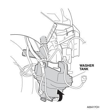
29. Secure the fog light harness to the vehicle harness with four wire ties. Do not secure the fog light harness to the washer tube.
