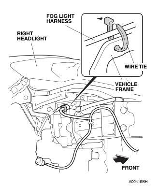
31. Route the fog light harness along the bumper beam as shown.
