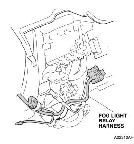
43. Attach the fog light relay harness relay block to the vehicle relay block.
