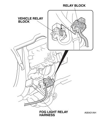
44. Unclip the vehicle connectors from the vehicle panel.
