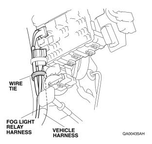
55. Unplug the vehicle connector from the combination light switch.
