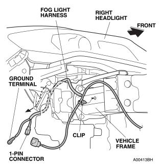
22. Secure the clip on the fog light harness to the vehicle frame as shown.
