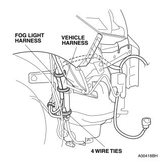
30. Secure the fog light harness to the vehicle frame with one wire tie as shown.
