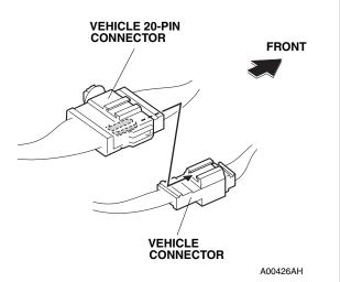
46. Remove the clip from the vehicle 20-pin connector, and install the supplied clip on the vehicle 20-pin connector.
