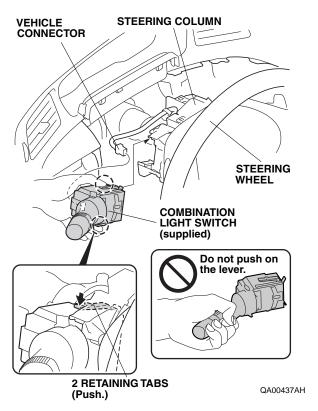
58. Plug the vehicle connector into the supplied combination light switch. Make sure the vehicle harness has some slack.
